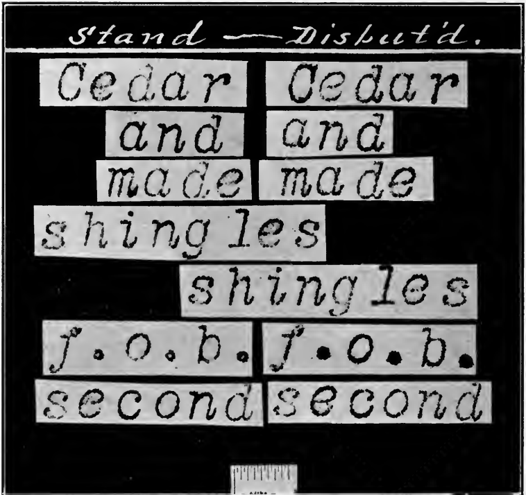
FIG. 201—From exhibits in case tried at Olean, N. Y., July, 1910. Standard typewriting on left, disputed on right.
